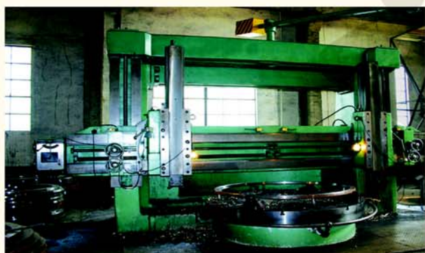
大型立车 Large vertical boring mill
